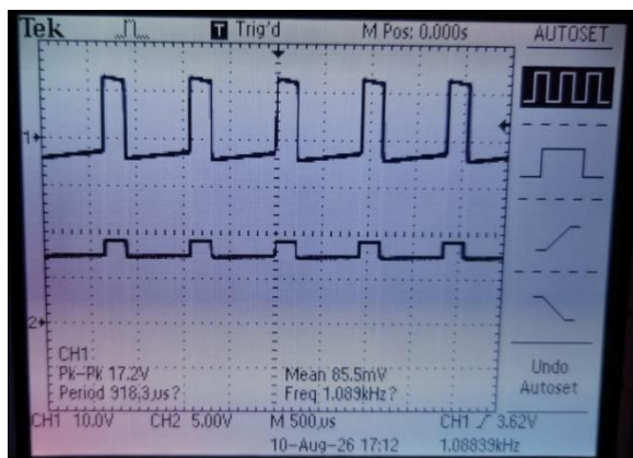
Fig. 16. Fuzz Face waveform response with VR1 adjusted to near 0kΩ
