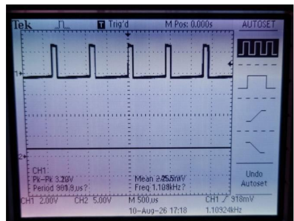
Fig. 18. Fuzz Face waveform response with 'Fuzz Pot' adjusted to near 0kΩ
